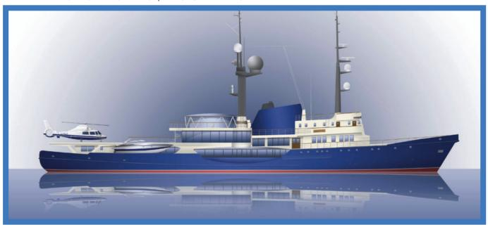
. Length Overall: 77.4 m . Main Engines: 2. x 4400 bhp . Propellers: 4. bladed CPP . Beam: 13.2 m . Draught: 5.78 m . Generators: 3. x 440kW . Cruising Speed: 15. kn . Bow Thruster: 1. x 400HP CPP
