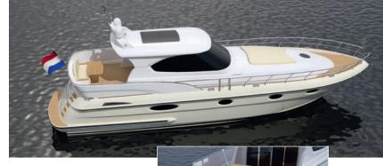
LOA: 56' Beam: 16' Draft: 3' Fuel: 634 Gal. Water: 214 Gal. Engines: 2 x Volvo Penta IPS 600, 435 hp Maximum speed: 20-24 knots
